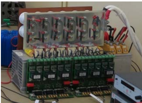
High precision switching amplifier with <-90dB zero crossing distortion
