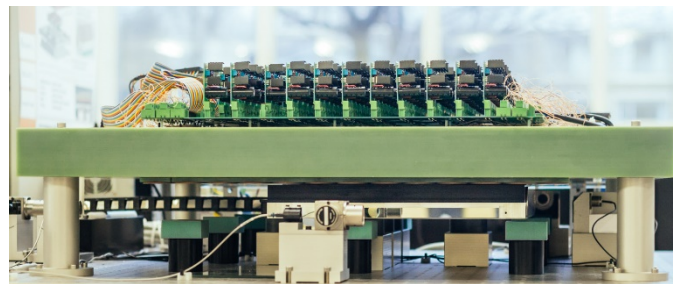
Ceiling robot with integrated wireless energy transfer
