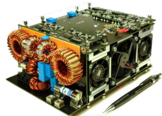
1-Phase bidirectional onboard charger with power density
