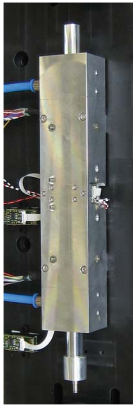
Integrated linear and rotary actuator for pick-and-place ( 150 \text{ m/s}^2 )
